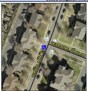
STROUD PARK CT Street 1 Name Stop Condition-Street 1 None Street 2 Name N/A Stop Condition-Street 2 N/A Possible Solutions: Remove & Replace Curb Ramp With **Two New Directional Ramps or** Equivalent. Surveyor Notes: N/A PROW/ADA:
