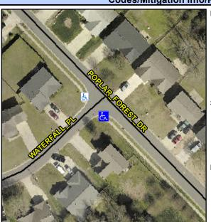
Street 1 Name Stop Condition-Street 2 Street 2 Name Stop Condition-Street 1 POPLAR FOREST DR None WATERFALL PL StopSign Possible Solutions: Remove & Replace Curb Ramp With Two New Directional Ramps or Equivalent. Surveyor Notes: N/A PROW/ADA: R304.5.1, R304.5.3
