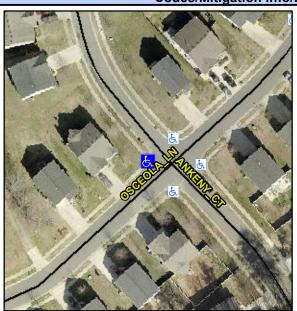
Street 1 Name Stop Condition-Street 2 Street 2 Name Stop Condition-Street 1 **OSCEOLA LN** None **ANKENY CT**  Possible Solutions: **Remove & Replace Curb Ramp With Two New Directional Ramps or** Equivalent.
