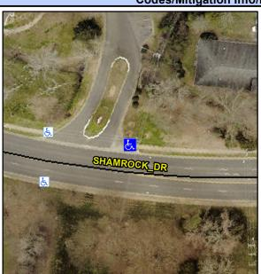
Street 1 Name **ENTRANCE** Stop Condition-Street 2 None SHAMROCK DR Street 2 Name Stop Condition-Street 1 None Possible Solutions: Remove & Replace Curb Ramp With Two New Directional Ramps or Equivalent. Surveyor Notes: N/A PROW/ADA: Not Found, R304.5.1, R304.2.2
