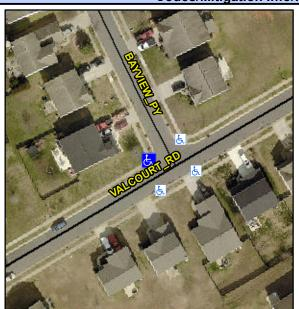
Street 1 Name Stop Condition-Street 2 Street 2 Name Stop Condition-Street 1 **VALCOURT RD** None **BAYVIEW PY** StopSign Possible Solutions: Remove & Replace Curb Ramp With **Two New Directional Ramps or** Equivalent. Surveyor Notes: N/A PROW/ADA: Not Found, R304.5.1, R304.5.3
