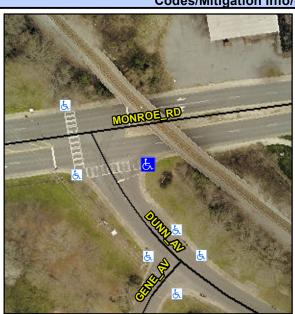
MONROE RD Street 1 Name Stop Condition-Street 2 Signal **DUNN AV** Street 2 Name Stop Condition-Street 1 Signal Possible Solutions: Remove & Replace Curb Ramp With **Two New Directional Ramps or** Equivalent. Surveyor Notes: N/A PROW/ADA: Not Found, R304.5.1, R304.2.2
