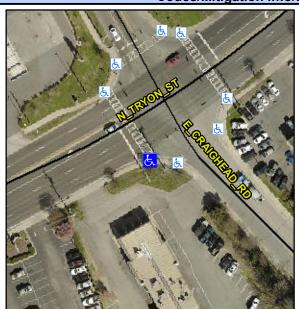
N TRYON ST Street 1 Name Stop Condition-Street 2 Signal Street 2 Name N/A Stop Condition-Street 1 N/A Possible Solutions: Remove & Replace Entire Ramp. Surveyor Notes: N/A PROW/ADA: Not Found, R304.5.1, R304.2.2, R304.5.3
