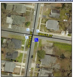
**GRACE ST** Street 1 Name Stop Condition-Street 1 StopSign **PEGRAM ST** Street 2 Name Stop Condition-Street 2 StopSign Possible Solutions: Remove & Replace Curb Ramp With Two New Directional Ramps or Equivalent. Surveyor Notes: N/A PROW/ADA: Not Found, R305.2, R302.7.2
