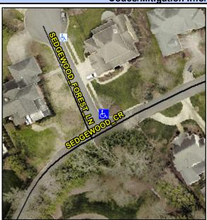
SEDGEWOOD FOREST LN Street 1 Name Stop Condition-Street 2 StopSign **SEDGEWOOD CR** Street 2 Name Stop Condition-Street 1 None Possible Solutions: Remove & Replace Curb Ramp With Two New Directional Ramps or Equivalent. Surveyor Notes: N/A PROW/ADA: R304.5.1
