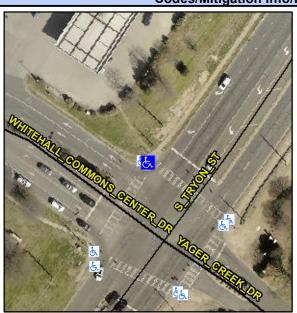
S TRYON ST Street 1 Name Stop Condition-Street 2 Signal Street 2 Name N/A Stop Condition-Street 1 N/A Possible Solutions: Remove & Replace Entire Ramp. Restripe Crosswalk. Surveyor Notes: N/A PROW/ADA: Not Found, R304.5.1, R304.2.2, R304.5.3
