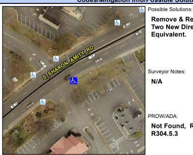
**S SHARON AMITY RD** Street 1 Name Stop Condition-Street 2 **ENTRANCE** Street 2 Name Stop Condition-Street 1 StopSign Remove & Replace Curb Ramp With Two New Directional Ramps or Equivalent.
