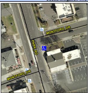
MONTFORD DR Street 1 Name Stop Condition-Street 2 StopSign Street 2 Name PARK RD Stop Condition-Street 1 None Possible Solutions: Remove & Replace Curb Ramp With **Two New Directional Ramps or** Equivalent. Surveyor Notes: N/A PROW/ADA: Not Found, R304.5.1, R304.2.2
