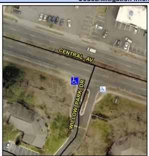
**WILLOW PARK DR** Street 1 Name Stop Condition-Street 1 None Street 2 Name N/A Stop Condition-Street 2 N/A Possible Solutions: Remove & Replace Curb Ramp With Two New Directional Ramps or Equivalent. Surveyor Notes: N/A PROW/ADA: Not Found, R304.5.1
