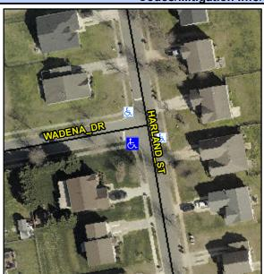
Street 1 Name Stop Condition-Street 2 Street 2 Name Stop Condition-Street 1 **HARLAND ST** StopSign **WADENA DR** StopSign Possible Solutions: Remove & Replace Curb Ramp With **Two New Directional Ramps or** Equivalent. Surveyor Notes: N/A PROW/ADA: Not Found, R304.2.2
