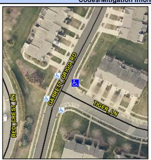
**GARRETT GRIGG RD** Street 1 Name Stop Condition-Street 2 None **TIGER LN** Street 2 Name Stop Condition-Street 1 StopSign Possible Solutions: Remove & Replace Curb Ramp With Two New Directional Ramps or Equivalent. Surveyor Notes: N/A PROW/ADA: Not Found, R304.5.1
