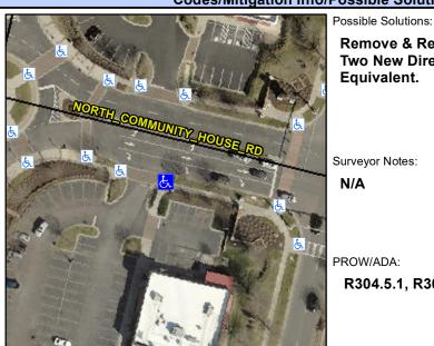
**COMMUNITY HOUSE RD** Street 1 Name Stop Condition-Street 2 YieldSign Street 2 Name **ENTRANCE** Stop Condition-Street 1 StopSign Remove & Replace Curb Ramp With Two New Directional Ramps or Equivalent.
