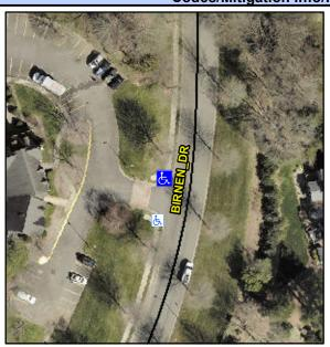
Street 1 Name Stop Condition-Street 2 Street 2 Name Stop Condition-Street 1 **ENTRANCE** None **BIRNEN DR**  Possible Solutions: Remove & Replace Curb Ramp With Two New Directional Ramps or Equivalent.
