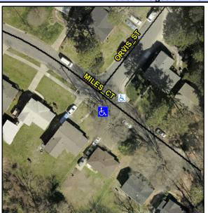
**MILES CT** Street 1 Name Stop Condition-Street 1 None Street 2 Name N/A Stop Condition-Street 2 N/A Possible Solutions: Remove & Replace Curb Ramp With **Two New Directional Ramps or** Equivalent. Surveyor Notes: N/A PROW/ADA: Not Found, R304.5.1, R304.5.3
