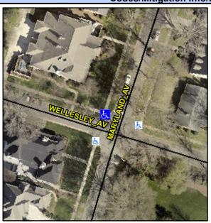
Street 1 Name Stop Condition-Street 2 Street 2 Name Stop Condition-Street 1 **WELLESLEY AV** None **MARYLAND AV** StopSign Possible Solutions: Remove & Replace Curb Ramp With Two New Directional Ramps or Equivalent.
