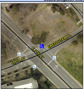
E 7TH ST Street 1 Name Stop Condition-Street 2 Signal Street 2 Name FIREFIGHTER PL Stop Condition-Street 1 Signal Possible Solutions: Remove & Replace Curb Ramp With **Two New Directional Ramps or** Equivalent. Surveyor Notes: N/A PROW/ADA: Not Found, R304.2.2, R304.5.3
