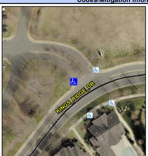
Street 1 Name Stop Condition-Street 2 Street 2 Name Stop Condition-Street 1 KINGS RIDGE DR None **ENTRANCE** StopSign Possible Solutions: Remove & Replace Curb Ramp With **Two New Directional Ramps or** Equivalent. Surveyor Notes: N/A PROW/ADA: Not Found, R304.2.2, R304.5.3
