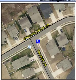
**HUBBARD FALLS DR** Street 1 Name Stop Condition-Street 2 **TOXAWAY CT** Street 2 Name Stop Condition-Street 1 StopSign Possible Solutions: Remove & Replace Curb Ramp With Two New Directional Ramps or Equivalent. Surveyor Notes: N/A
