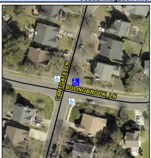
**CARTGATE LN** Street 1 Name Stop Condition-Street 2 StopSign **BOILINGBROOK LN** Street 2 Name Stop Condition-Street 1 None Possible Solutions: Remove & Replace Curb Ramp With Two New Directional Ramps or Equivalent. Surveyor Notes: N/A PROW/ADA: R304.2.2
