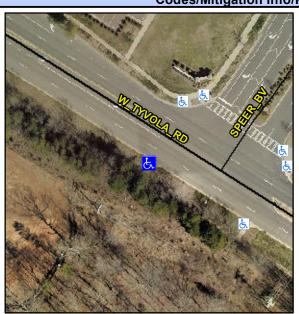
W TYVOLA RD Street 1 Name Stop Condition-Street 2 None N/A Street 2 Name Stop Condition-Street 1 N/A Possible Solutions: Remove & Replace Entire Ramp. Surveyor Notes: N/A PROW/ADA: Not Found, R304.2.2-Perp, R304.3.2-Para
