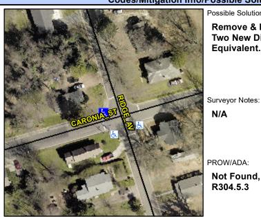
Street 1 Name Stop Condition-Street 2 Street 2 Name Stop Condition-Street 1 Possible Solutions: Remove & Replace Curb Ramp With Two New Directional Ramps or Equivalent.
