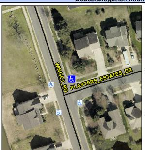
WINGET RD Street 1 Name Stop Condition-Street 2 Street 2 Name **PLANTERS ESTATES DR** Stop Condition-Street 1 StopSign Possible Solutions: Remove & Replace Curb Ramp With Two New Directional Ramps or Equivalent. Surveyor Notes: N/A PROW/ADA: Not Found, R305
