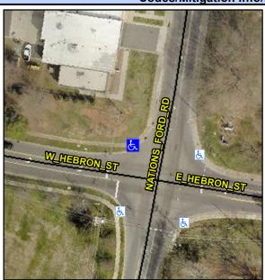
**E HEBRON ST** Street 1 Name Stop Condition-Street 2 Signal Street 2 Name **NATIONS FORD RD** Stop Condition-Street 1 Signal Possible Solutions: **Remove & Replace Curb Ramp With Two New Directional Ramps or** Equivalent. Surveyor Notes: N/A PROW/ADA: Not Found, R304.5.1, R304.5.3
