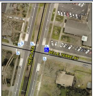
**BELLE TERRE AV** Street 1 Name Stop Condition-Street 1 StopSign Street 2 Name N/A Stop Condition-Street 2 N/A Possible Solutions: Remove & Replace Entire Ramp. Surveyor Notes: N/A R304.2.2
