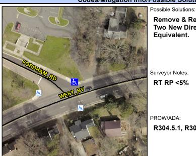
**FORDHAM RD** Street 1 Name Stop Condition-Street 1 StopSign **WEST BV** Street 2 Name Stop Condition-Street 2 None Remove & Replace Curb Ramp With Two New Directional Ramps or Equivalent.
