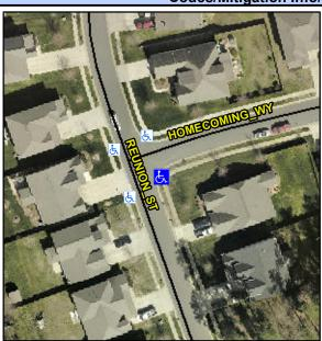
Street 1 Name **HOMECOMING WY** Stop Condition-Street 2 StopSign **REUNION ST** Street 2 Name Stop Condition-Street 1 None Possible Solutions: Remove & Replace Curb Ramp With Two New Directional Ramps or Equivalent. Surveyor Notes: N/A PROW/ADA: R304.2.2
