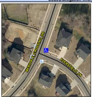
Street 1 Name Stop Condition-Street 2 Street 2 Name Stop Condition-Street 1 MERIDALE CROSSING DR None **EVERSFIELD LN** StopSign Possible Solutions: Remove & Replace Curb Ramp With **Two New Directional Ramps or** Equivalent. Surveyor Notes: N/A PROW/ADA: R304.2.2, R304.5.3
