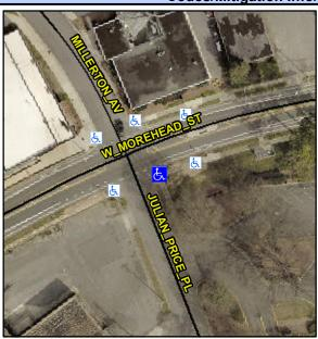
Street 1 Name Stop Condition-Street 2 Street 2 Name Stop Condition-Street 1 W MOREHEAD ST None **JULIAN PRICE PL** StopSign Possible Solutions: Remove & Replace Curb Ramp With **Two New Directional Ramps or** Equivalent. Surveyor Notes: N/A PROW/ADA: Not Found, R304.2.2, R304.5.3
