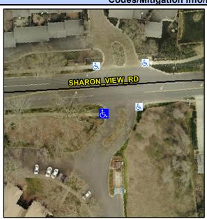
**ENTRANCE** Street 1 Name Stop Condition-Street 2 None **SHARON VIEW RD** Street 2 Name Stop Condition-Street 1 None Possible Solutions: Remove & Replace Curb Ramp With Two New Directional Ramps or Equivalent. Surveyor Notes: N/A PROW/ADA: R304.5.1
