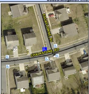
**CHALKSTONE RD** Street 1 Name Stop Condition-Street 2 None Street 2 Name **ESCAFLOWNE AV** Stop Condition-Street 1 StopSign Possible Solutions: **Remove & Replace Curb Ramp With Two New Directional Ramps or** Equivalent. Surveyor Notes: N/A PROW/ADA: Not Found, R304.5.1, R304.5.3
