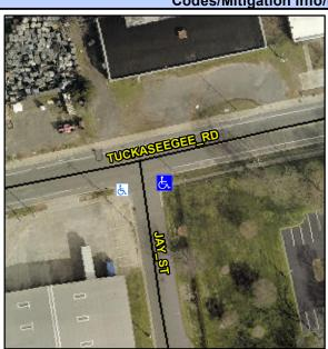
**TUCKASEEGEE RD** Street 1 Name Stop Condition-Street 2 None **JAY ST** Street 2 Name Stop Condition-Street 1 StopSign Possible Solutions: Compliance Description Remove & Replace Curb Ramp With Two New Directional Ramps or Equivalent. Surveyor Notes: N/A PROW/ADA: Not Found, R304.2.2, R304.5.3
