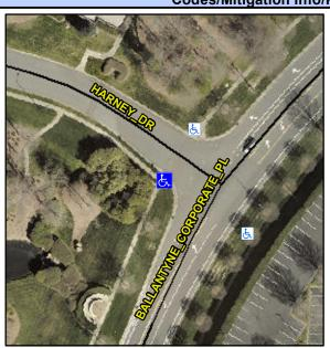
**BALLANTYNE CORPORATE PL** Street 1 Name Stop Condition-Street 2 None **HARNEY DR** Street 2 Name Stop Condition-Street 1 StopSign Possible Solutions: Remove & Replace Curb Ramp With Two New Directional Ramps or Equivalent. Remove & Replace Gutter. Surveyor Notes:
