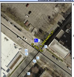
E 3RD ST Street 1 Name Stop Condition-Street 2 Signal Street 2 Name N/A Stop Condition-Street 1 N/A Possible Solutions: Remove & Replace Entire Ramp. Surveyor Notes: N/A PROW/ADA: Not Found, R304.5.1, R304.5.3
