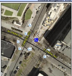
**CAMDEN RD** Street 1 Name Stop Condition-Street 2 Signal **E PARK AV** Street 2 Name Stop Condition-Street 1 Signal Possible Solutions: Remove & Replace Curb Ramp With Two New Directional Ramps or Equivalent. Surveyor Notes: N/A PROW/ADA: R304.5.1
