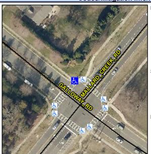
**GALLOWAY RD** Street 1 Name Stop Condition-Street 2 Signal Street 2 Name N/A Stop Condition-Street 1 N/A Possible Solutions: Remove & Replace Entire Ramp. Surveyor Notes: N/A PROW/ADA: R304.5.1, R304.2.2
