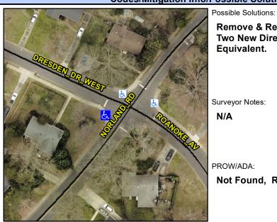
**ROANOKE AV** Street 1 Name Stop Condition-Street 1 StopSign Street 2 Name N/A Stop Condition-Street 2 N/A Remove & Replace Curb Ramp With **Two New Directional Ramps or** Equivalent.
