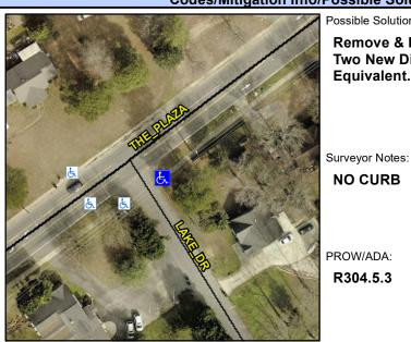
LAKE DR Street 1 Name Stop Condition-Street 1 StopSign Street 2 Name N/A Stop Condition-Street 2 N/A Possible Solutions: Remove & Replace Curb Ramp With **Two New Directional Ramps or** Equivalent.
