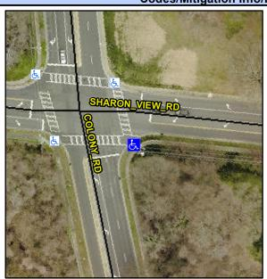
**SHARON VIEW RD** Street 1 Name Stop Condition-Street 2 Signal **COLONY RD** Street 2 Name Stop Condition-Street 1 Signal Possible Solutions: Remove & Replace Curb Ramp With Two New Directional Ramps or Equivalent. Surveyor Notes: N/A PROW/ADA: R304.5.1, R304.2.2, R304.5.3
