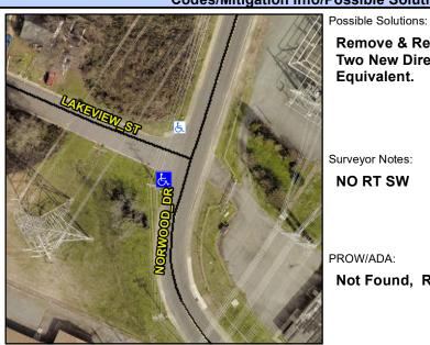
**LAKEVIEW ST** Street 1 Name Stop Condition-Street 1 StopSign Street 2 Name N/A Stop Condition-Street 2 N/A Remove & Replace Curb Ramp With Two New Directional Ramps or Equivalent.
