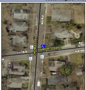
**THOMAS AV** Street 1 Name Stop Condition-Street 2 None Street 2 Name **HAMORTON PL** Stop Condition-Street 1 StopSign Possible Solutions: Remove & Replace Curb Ramp With **Two New Directional Ramps or** Equivalent. Surveyor Notes: N/A PROW/ADA: Not Found, R304.5.1, R304.2.2, R304.5.3
