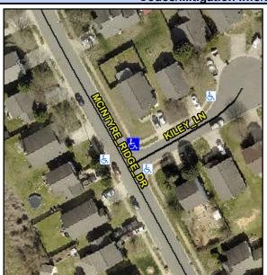
**KILEY LN** Street 1 Name Stop Condition-Street 2 None Street 2 Name MCINTYRE RIDGE DR Stop Condition-Street 1 StopSign Possible Solutions: Remove & Replace Curb Ramp With Two New Directional Ramps or Equivalent. Surveyor Notes: N/A PROW/ADA: Not Found, R304.5.3
