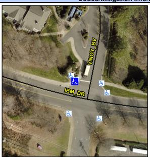
Street 1 Name Stop Condition-Street 1 IBM DR Street 2 Name StopSign Stop Condition-Street 2 VINOY BV Possible Solutions: Remove & Replace Curb Ramp With Two New Directional Ramps or Equivalent. Remove & Replace Sidewalk. Surveyor Notes: N/A PROW/ADA: Not Found, R304.5.1, R304.3.2
