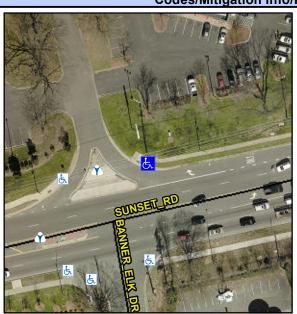
**SUNSET RD** Street 1 Name Stop Condition-Street 1 None N/A Street 2 Name Stop Condition-Street 2 N/A Possible Solutions: Remove & Replace Curb Ramp With Two New Directional Ramps or Equivalent. Surveyor Notes: N/A PROW/ADA: Not Found, R304.5.1
