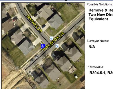
Street 1 Name Stop Condition-Street 2 Street 2 Name Stop Condition-Street 1 TWIN BROOK DR None MINTVALE DR StopSign Remove & Replace Curb Ramp With Two New Directional Ramps or Equivalent.
