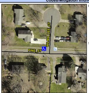
**WILMA LEE CT** Street 1 Name Stop Condition-Street 1 StopSign Street 2 Name N/A Stop Condition-Street 2 N/A Possible Solutions: Remove & Replace Curb Ramp With Two New Directional Ramps or Equivalent. Surveyor Notes: N/A PROW/ADA:
