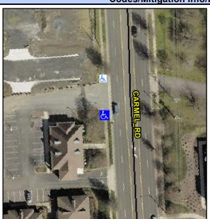
**CARMEL RD** Street 1 Name Stop Condition-Street 2 None **ENTRANCE** Street 2 Name Stop Condition-Street 1 StopSign Possible Solutions: Remove & Replace Curb Ramp With **Two New Directional Ramps or** Equivalent. Surveyor Notes: N/A PROW/ADA: Not Found, R304.2.2
